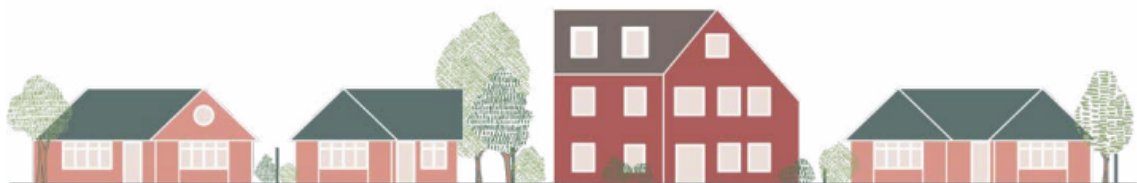
Figure 2.10d: Where surrounding buildings are predominantly single storey, new development should seek to accommodate a third storey within the roof space.
